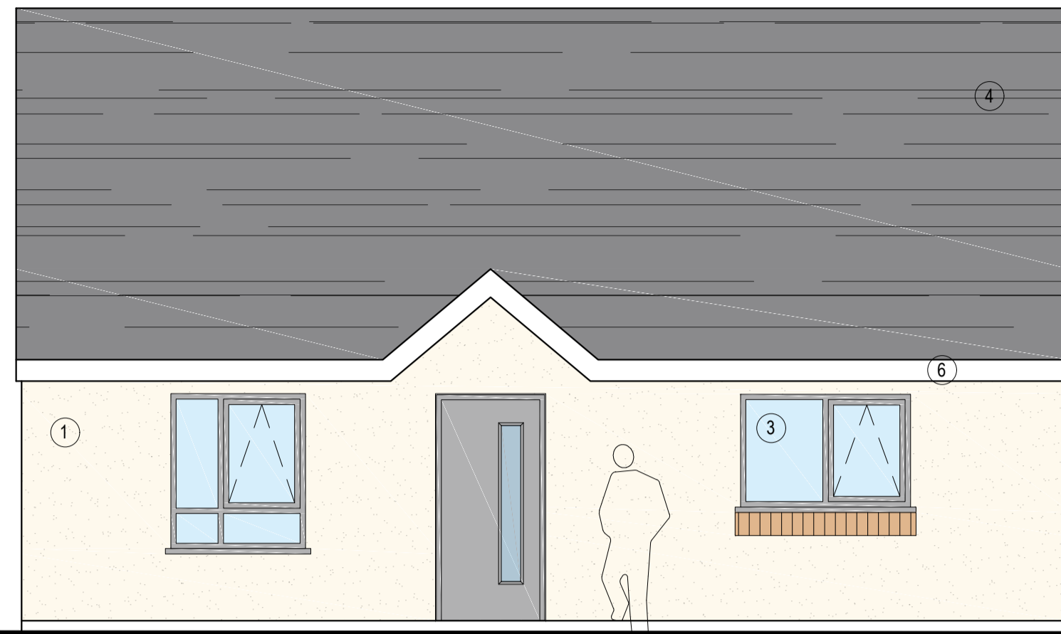
Front Elevation (Render alternative) Scale 1:50
